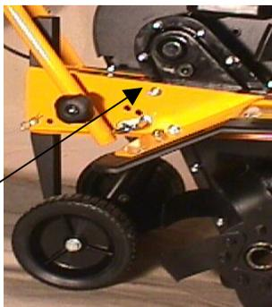
The gearbox on the tiller is from the factory lubricated with 0.2 litre TEXACO Multifak 283 EPOO oil. It is not necessary to renew the oil
