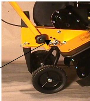
The supportwheels are mounted on the tiller. The adjustment is done by means of the lock . Pull the lock out, and lift or lower the tiller with the handlebar until the preferred height is found. Release the lock.
